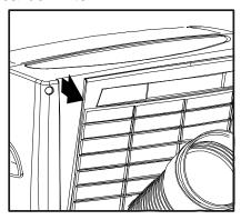
1. Shut off the unit. Pull the pre-filter towards the hose.
